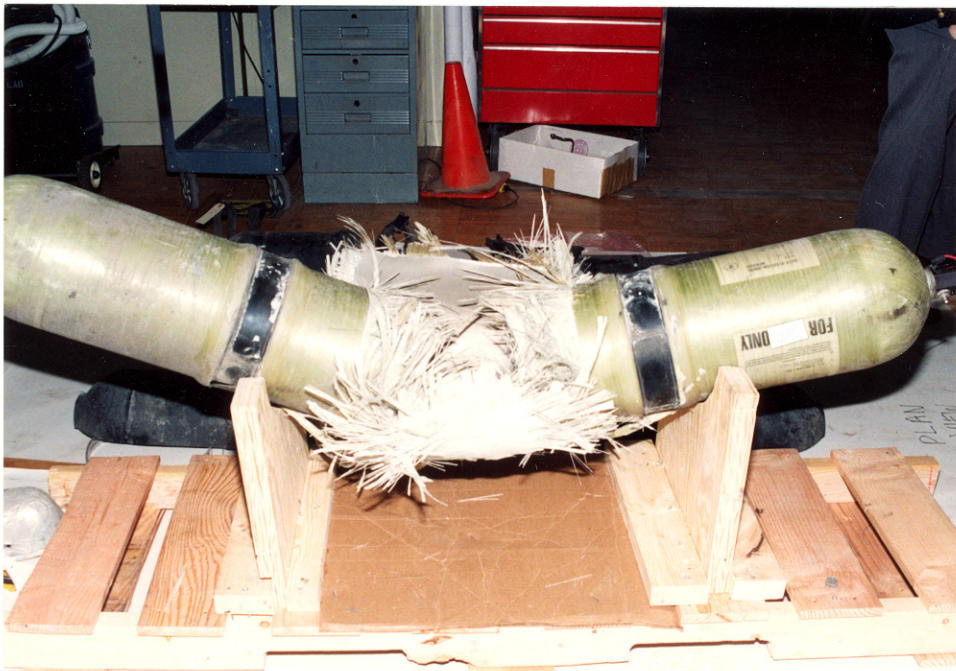
38. View of the failed CNG tank with the bottom of the tank as mounted in the vehicle shown facing up in the photograph and the forward end along the right side of the photograph
